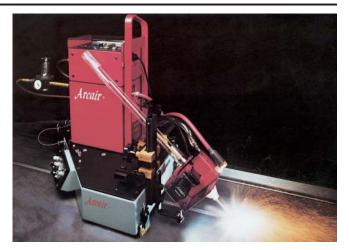
Groove depth is maintained within a tolerance  $\pm 0.025$ " (0,635mm). The N6000 System is ideally suited for metal fabrication, particularly in weld joint preparation, where it is used to prepare uniform "U" or "J" grooves. The System is also used extensively for backgouging of seams and for removing defective welds and cracks.
