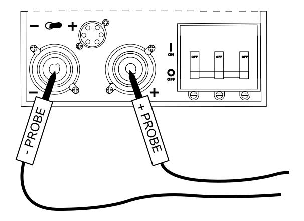
5. If 200 ohms is measured then the output diodes are not "shorted".
