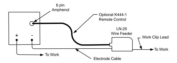
**NOTE:** Illustation shows electrode connected for negative polarity.
