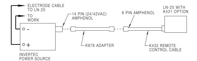
**NOTE**: Illustration shows electrode connected for positive polarity.
