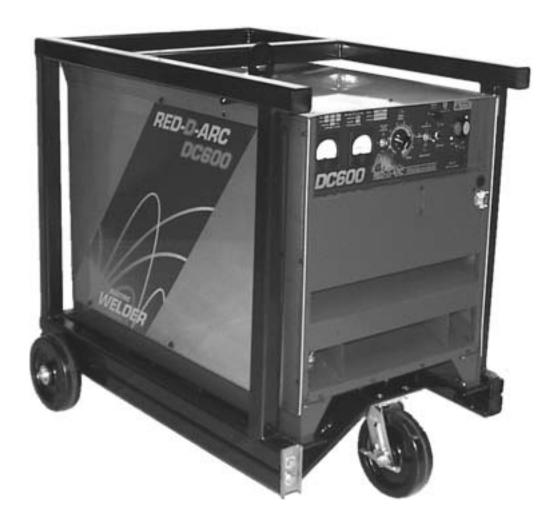
Rugged Tubular Pak-Lok-Frame<sup>™</sup> Extreme-Duty<sup>™</sup> Stainless Steel Construction 600 amps DC at 44 volts and 100% Duty Cycle Available in 4Pak<sup>™</sup> Multioperator Systems and in Selecta-Paks<sup>™</sup> for Multiprocess Applications
